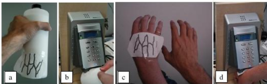
Figure 4-10. Spoof for Techsphere (Back of Hand) Vein Scanner
